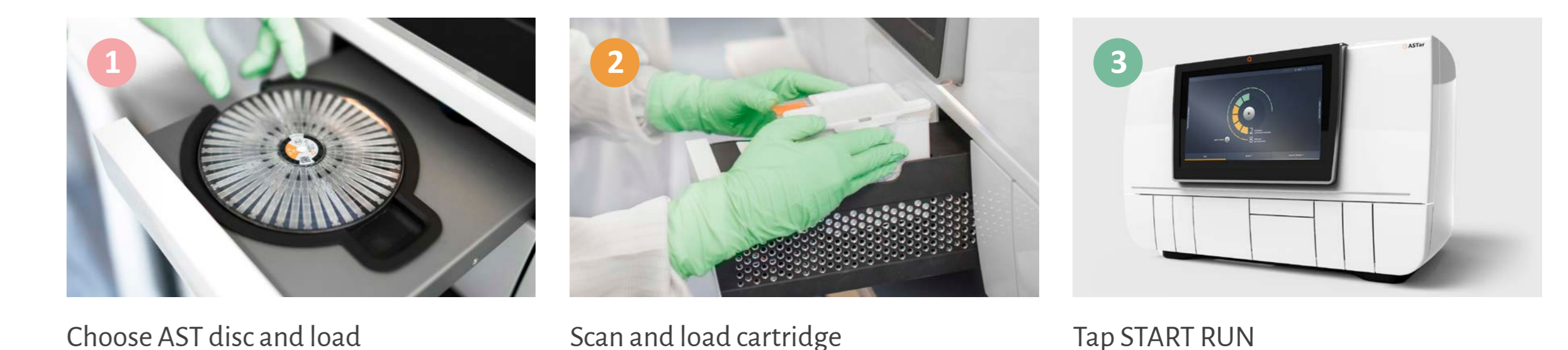
Fig 2. Workflow to load and run a sample in the fully automated system used in the study.
